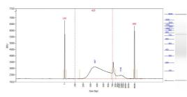
Figure 6 An example of an over-tagmented library profile with a peak at 187 bp and an adapter peak at 42 bp
